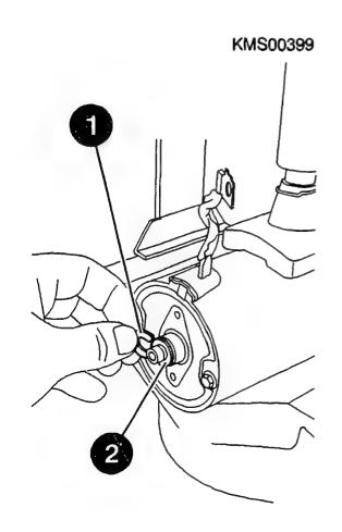
Disassembling commutator end shield Unfasten bolts (1).
